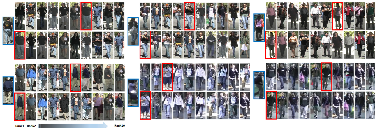
Fig. 2. The improvement of ranking result by our OLMANS on VIPeR [36]. BLUE boxes: input probes, RED: gallery targets. For each case, the top row is the result from the baseline [5], and the bottom row is our result. (Best view in color and enlarged).
