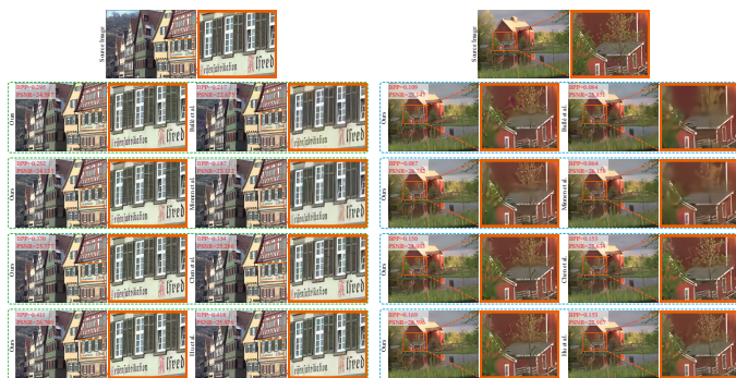
Fig. 8: Visualization of sample images in Kodak dataset. Compared with single-rate methods (Ballé et al. [10], Minnen et al. [29], Chen et al. [36]), and Hu et al. [32] which need multiple models to achieve different compression rates. For each comparison, we adjust the bpp of our I2C to adapt those methods. Our I2C has much better fidelity-preserving performance and is a variable-rate method.
